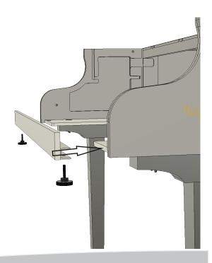
Fully tighten the sled hardware from the earlier step.
